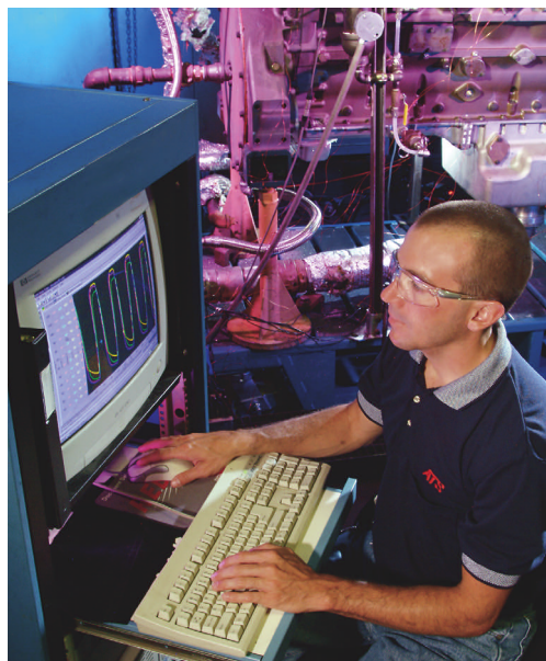
A Caterpillar test engineer runs diagnostic tests measuring engine exhaust particulates. Courtesy of Caterpillar.
